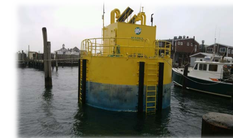
Automated Feed Buoy powered by Solar and diesel back-up generator holds up to 20 tons of feed.
